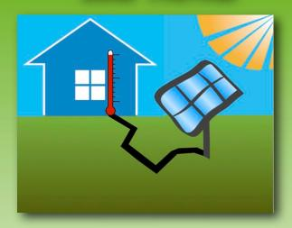
Solar Thermal Systems collect sunlight and turn it into thermal energy or heat. The heat is then pumped into a storage tank for later use. That heat can then be used for many purposes, including:
